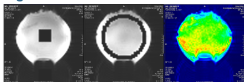
Figure 1: Central slice of the phantom containing the central ROI (left), the peripheral ROI (center) and detrended tSNR map computed on a pixel-by-pixel basis.
